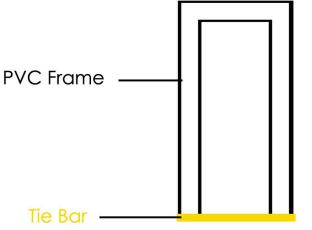
The first process is to insert a fixing material into the and of the profile which the tie bar can then be attached to, a piece of timber (not supplied) 100mm in length should be sufficient
